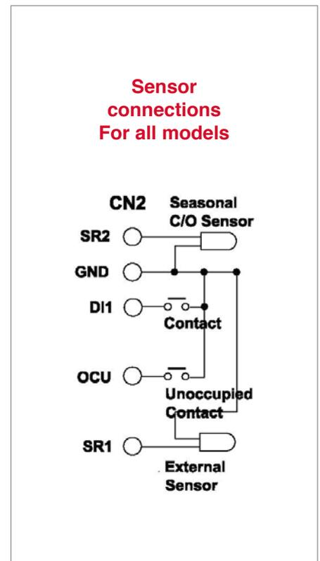
**WARNING:** Incorrect wiring connection may cause permanent equipment damages to the thermostat
