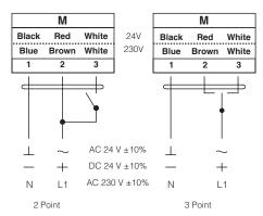
↑ Connect via safety isolating transformer
