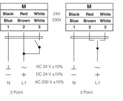
A Connect via safety isolating transformer
