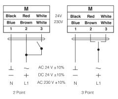
↑ Connect via safety isolating transformer
